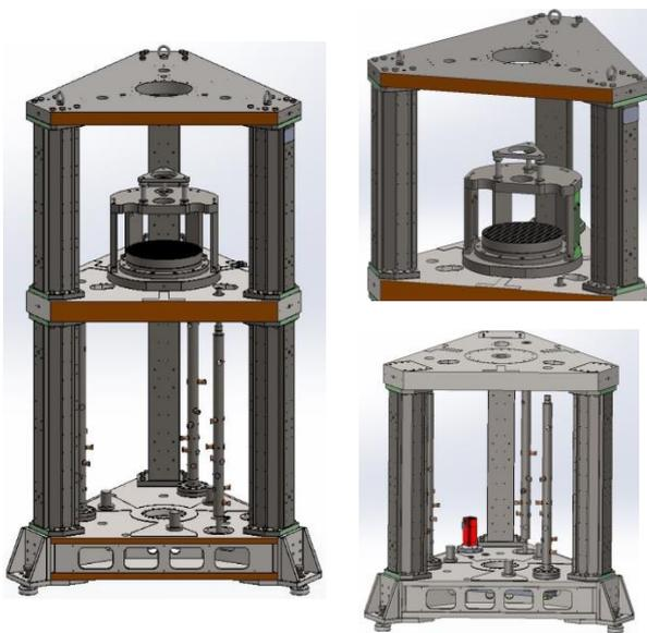
Figure 5: High Load Brinell Hardness Standard Machine
