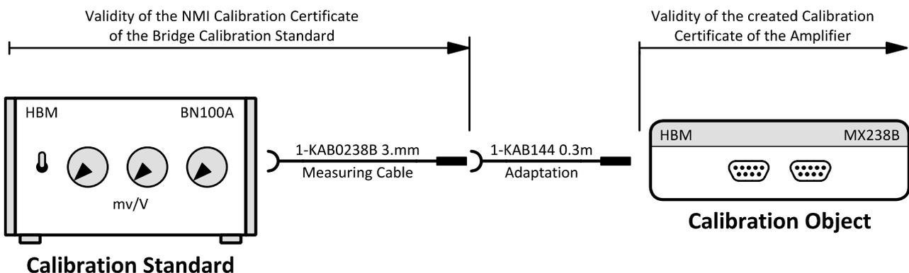
Figure 1: Setup of measurement for calibration of the MX238B
