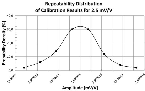
Figure 7: Repeatability distribution of calibration results
