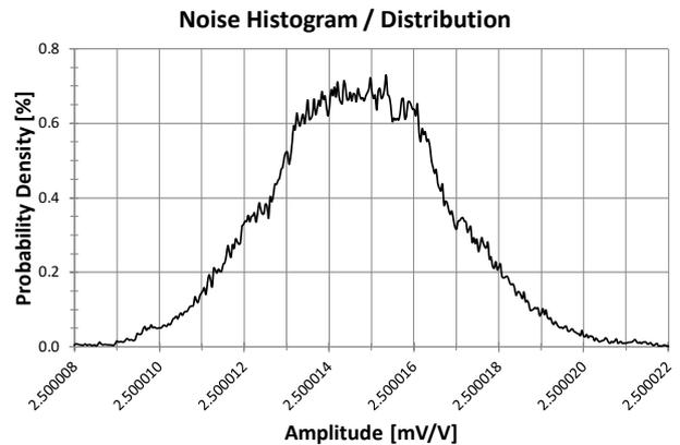
Figure 6: Noise histogram for a combination of MX238B and BN100A
