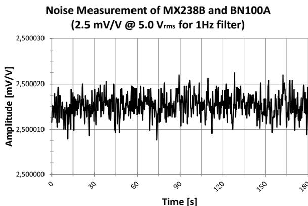
Figure 5: Noise measurement for a combination of MX238B and BN100A
