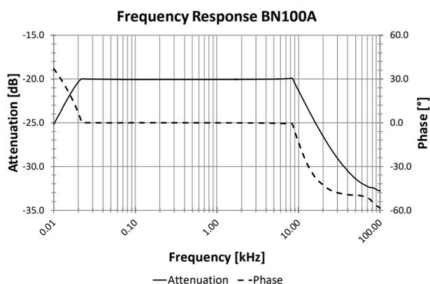
Figure 4: Frequency response of the BN100A
