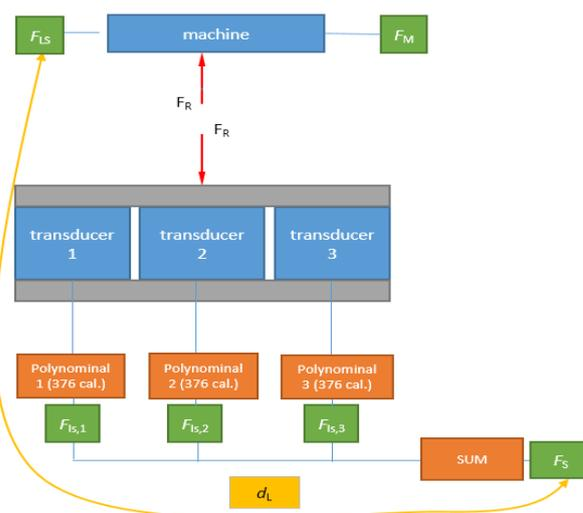
Figure 6: Signal generation from the real acting force to the measured sum force [10]
