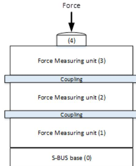
Figure 3: The schematic drawing of the proposed design of the S-BUS
