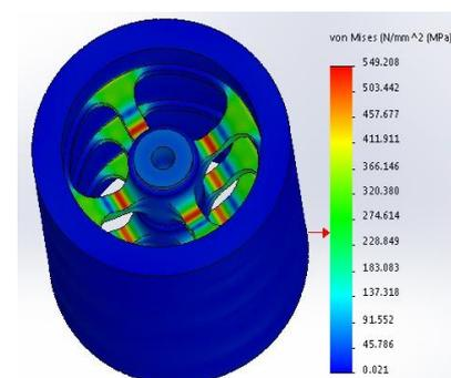
Figure 5: FE results for S-BUS model (30 kN force)
