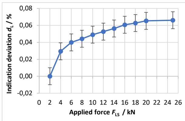
Figure 10: The 30 kN S-BUS indication deviation
