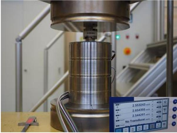
Figure 8: Calibration of the 30 kN S-BUS on the 100 kN PTB D-FSM
