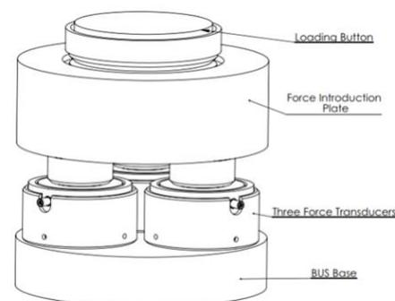
Figure 1: A schematic drawing of the P-BUS
