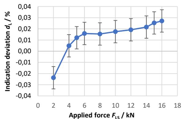
Figure 9: The 20 kN S-BUS indication deviation
