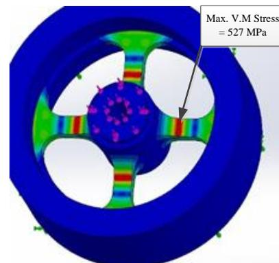
Figure 4: FE results for Single transducer Model (10 kN force)
