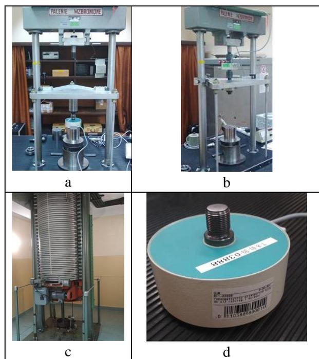
Figure 1: GUM's force reference standard maintained at the Central Office of Measures through application of the force standard machine No. S03 (WS-55 kN), covering the force range from 1 kN up to 55 kN, with the uncertainty of applied force 0.01 % of the measured value: a) upper part: FSM with mounted force transducer prepared for compressive test; b) upper part: FSM with mounted force transducer prepared for tension test; c) FSM - lower part; d) HBM Z4A force transducer
