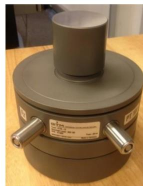
Figure 2: Force transducer with PT100 inside
