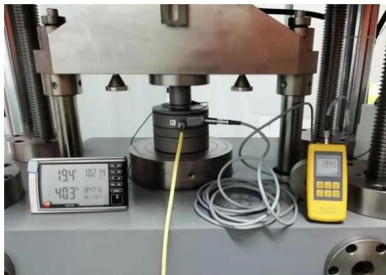
Figure 3: Temperature measurement
