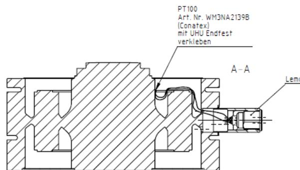
Figure 1: PT100 inside the transducer
