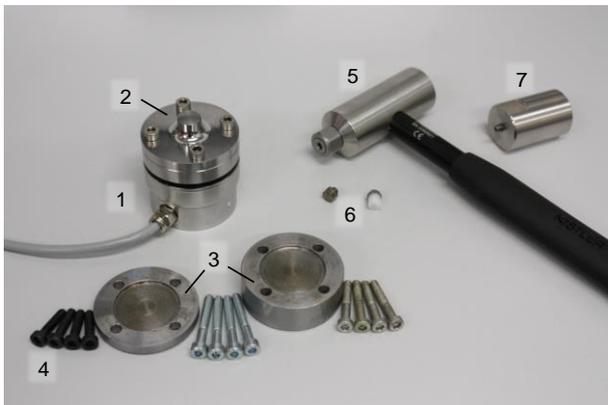
Figure 6: Components of the calibration experiments: HBM U3/10 kN force transducer (1) with load adapter (2) and two optional load mass discs (3) plus mounting screws (4); Kistler 9726A20000 impact hammer (5) with two hammer tips (6) and optional mass extender (7).
