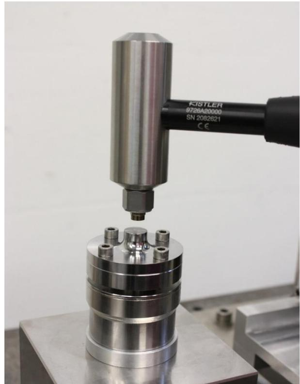
Figure 7: In-situ dynamic force calibration using a load mass of 135 g and a steel hammer tip.
