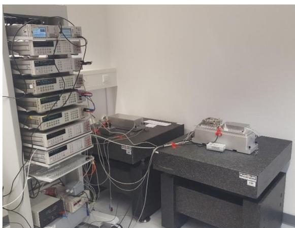
Figure 1: The PB2 set-up: balance and interferometer (right) and signal processing system (left).
