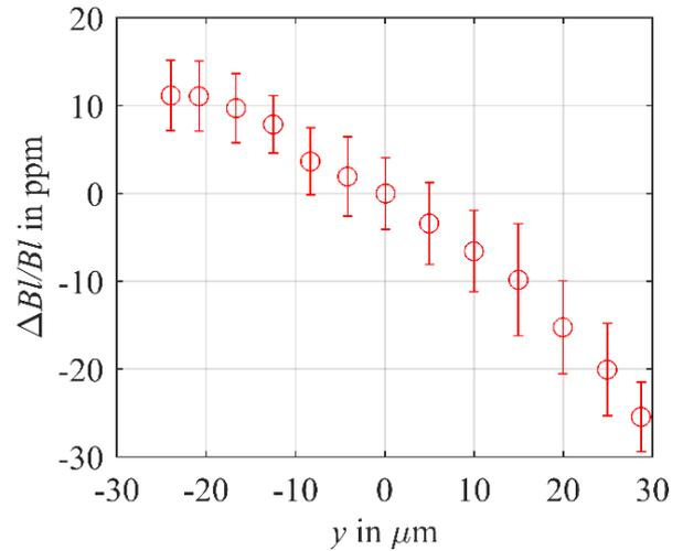
Figure 4: Relative change of  $Bl$  depending on coil position.
