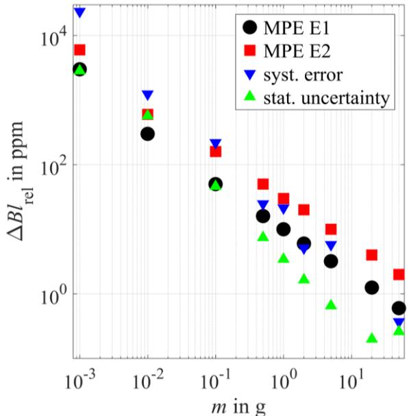
Figure 7: Deviation between force and velocity mode.
