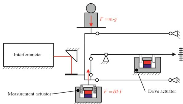
Figure 2: Schematic of the PB2 set-up.
