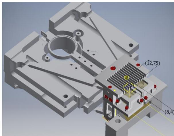
Figure 3: CAD model of the weighing cell mechanics and the weighing pan with fork structure.
