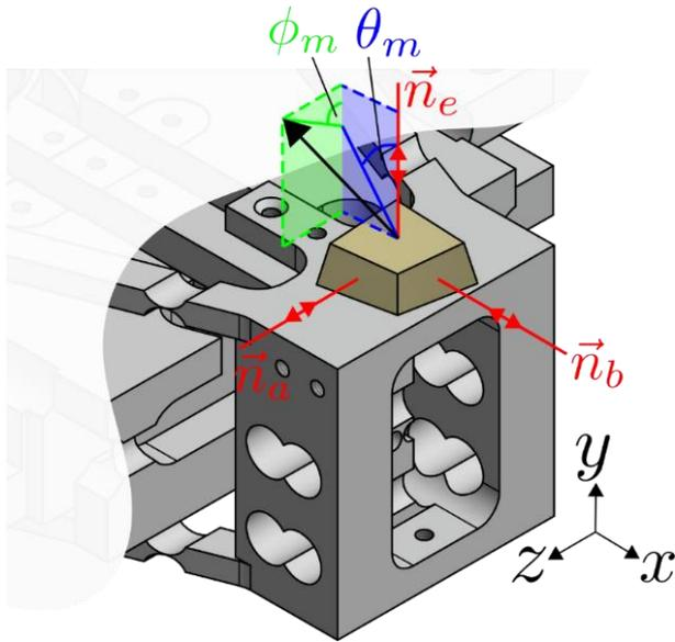
Figure 5: Schematic of the alignment axes with an alignment cuboid.
