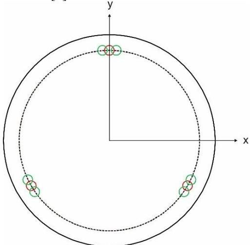
Figure 2: Top view of the location of the spherical distance pieces of a gap between two discs. Green marked spheres are fixed on the lower disc, red labelled spherical distance pieces are located on the upper disc.
