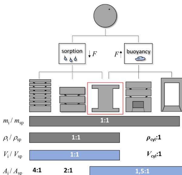
Figure 1: Schematic illustration of ratios of different sorption artefacts (left), buoyancy artefacts (right), duplex artifact (middle, red)
