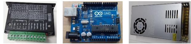
Figure 8: TB6600 stepper motor driver (at left), Arduino UNO R3 board (at the centre) and 24 V DC power supply (at right).
