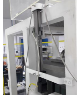
Figure 2: Overview of the automated mechanism designed for the handling of standard substitution weights implemented in IPQ's hydrostatic weighing apparatus.
