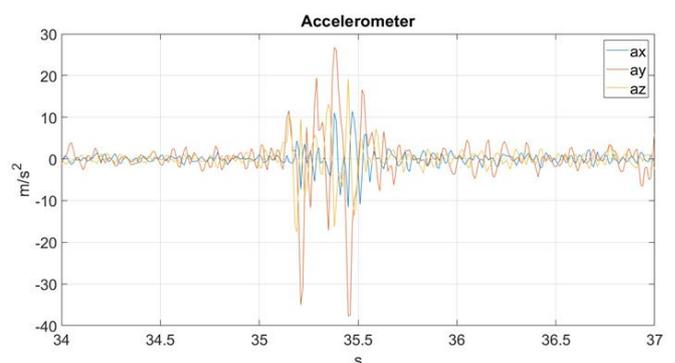
Figure 5. Spike in the acceleration signal due to a bump.
