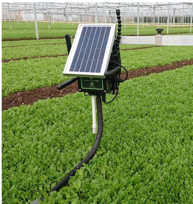
Figure 1. The appearance of an EVJA sensor node.
