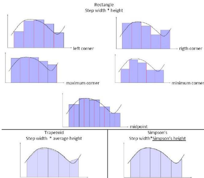
Figure 3. The numerical integration methods analysed in [19].
