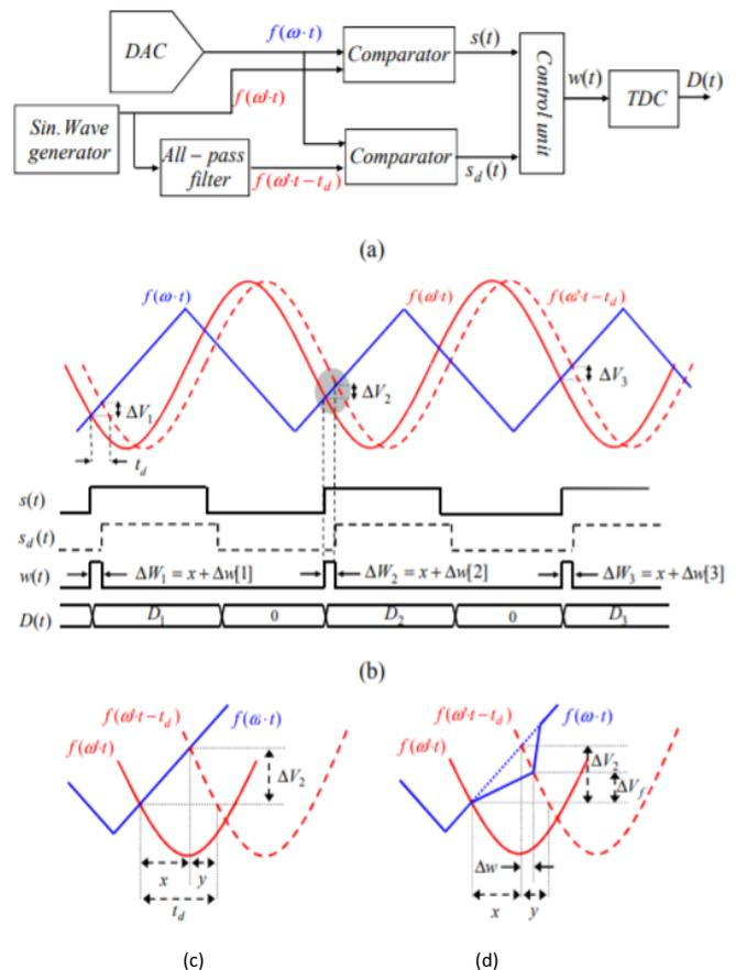
Figure 1. (a) The scheme of the proposed method with the dual undersampling technique. (b) The relative signals. (c) The shadow area in Figure 1 (b) of the linear case. (d) The shadow area in Figure 1 (b) of the non-linear case [14].
