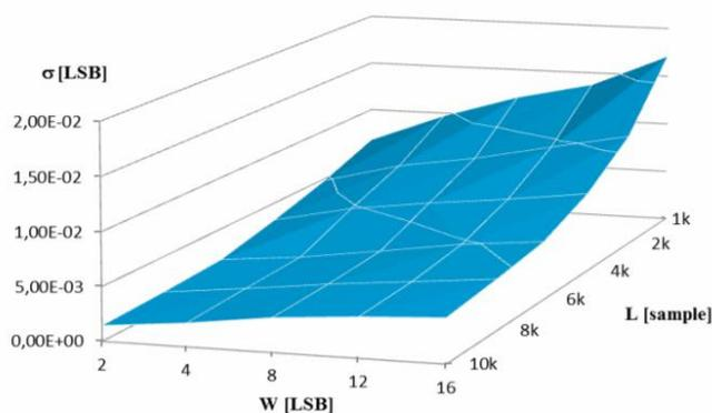
Figure 5. Dependence of the standard deviation of difference between the INL characteristics on the amplitude of dithering  $W$  and different numbers of samples  $L$  [39].
