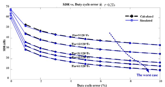
Figure 4. Simulated and calculated SDR changes with the duty cycle error at output time constant  $\tau = 0.2T_s$  [21].
