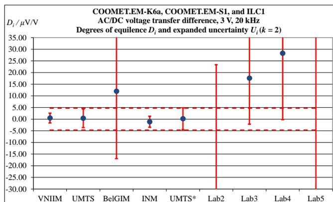
Figure 2. Degrees of equivalence of all laboratories for COOMET.EM-K6.a, COOMET.EM-S1 comparisons and ILC1 in terms of  $RV_{K6.a}$  at frequency of 20 kHz
