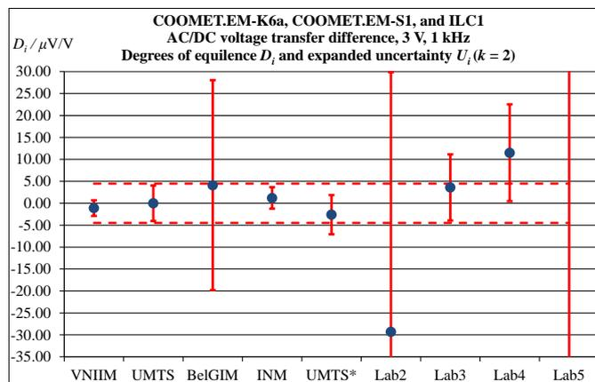
Figure 1. Degrees of equivalence of all laboratories for COOMET.EM-K6.a, COOMET.EM-S1 comparisons and ILC1 in terms of  $RV_{K6.a}$  at frequency of 1 kHz.
