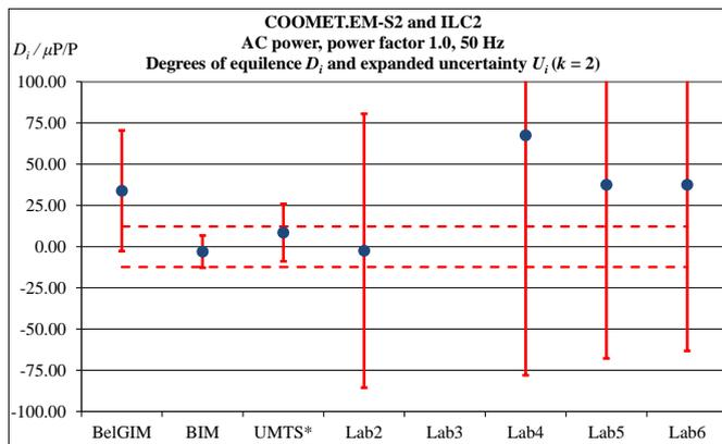
Figure 4. Degrees of equivalence of all laboratories for COOMET.EM-S2 comparisons and ILC2 in terms of  $RV_{S2}$  for power factor = 1.0.
