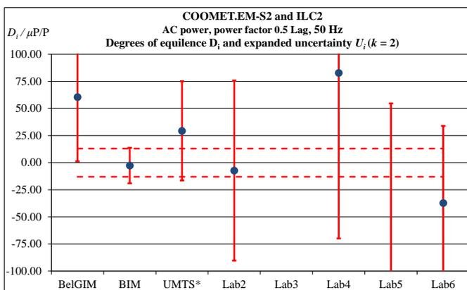
Figure 5. Degrees of equivalence of all laboratories for COOMET.EM-S2 comparisons and in ILC2 in terms of  $RV_{S2}$  for power factor = 0.5 Lag.
