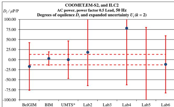
Figure 6. Degrees of equivalence of all laboratories for COOMET.EM-S2 comparisons and ILC2 in terms of  $RV_{S2}$  for power factor = 0.5 Lead.
