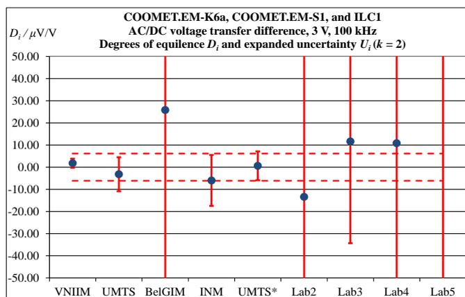
Figure 3. Degrees of equivalence of all laboratories for COOMET.EM-K6.a, COOMET.EM-S1 comparisons and ILC1 in terms of  $RV_{K6.a}$  at frequency of 100 kHz.
