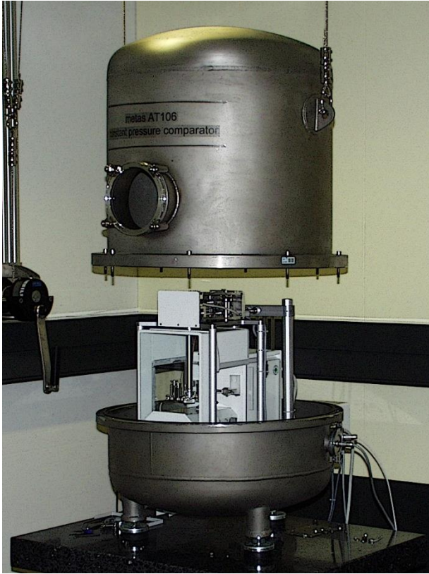
Figure 3. AT106 mass comparator with an airtight enclosure in the mass laboratory at METAS.
