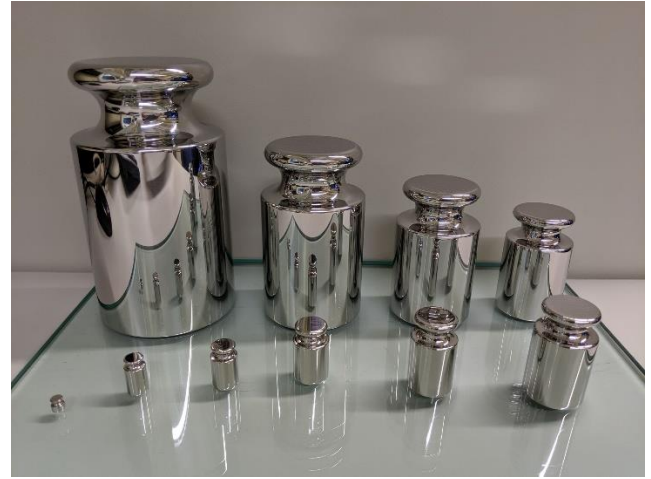
Figure 4. OIML stainless steel weights used for the comparison.
