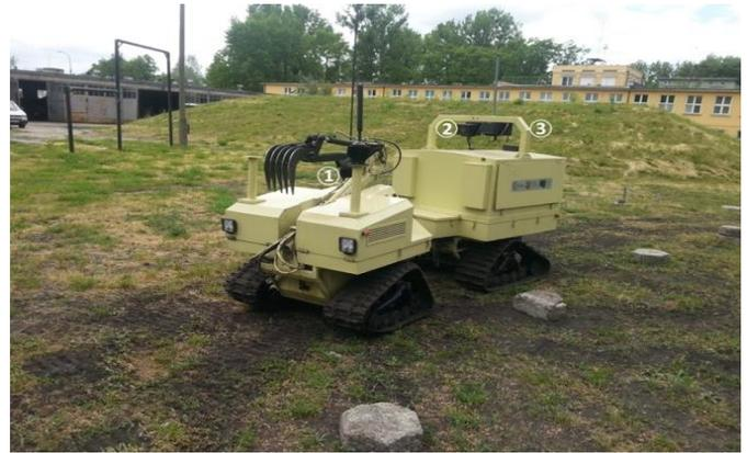
Figure 2. The DROMADER robot's cameras marked as 1, 2, and 3.
