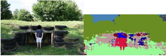
Figure 11. ENet's semantic segmentation output image of a lost person in front of a tunnel. Visual image frame from the child UAV (left), ENet segmentation of the image frame (red=victim).
