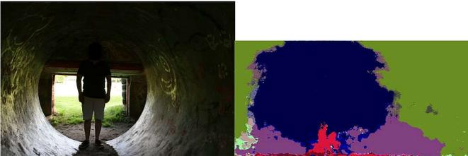
Figure 12. ENet's semantic segmentation output image of a lost person inside a tunnel. Visual image frame from the child UAV (left), ENet segmentation of the image frame (red=victim) (right)
