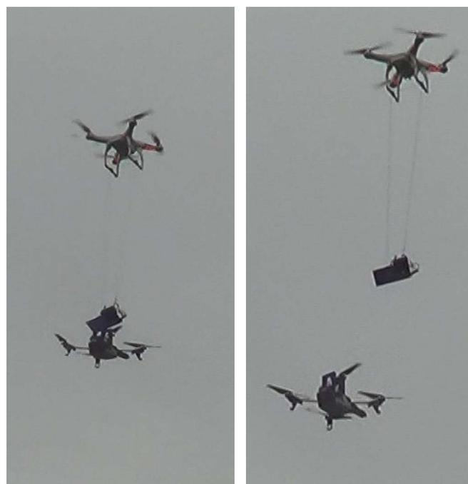
Figure 6. In-flight launch of the child UAV by the mothership UAV: UAVs before launch (left); UAVs after launch (right).
