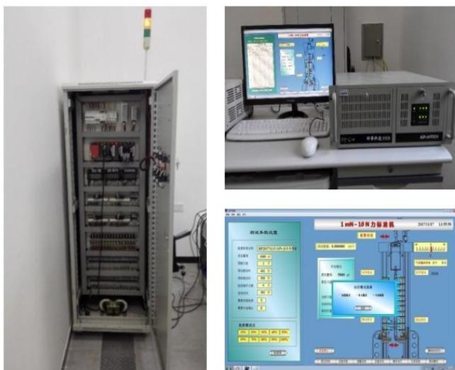
Figure 5. The electronic and control system.
