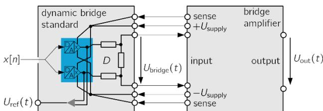
Figure 2. Schematic overview of the dynamic bridge standard.
