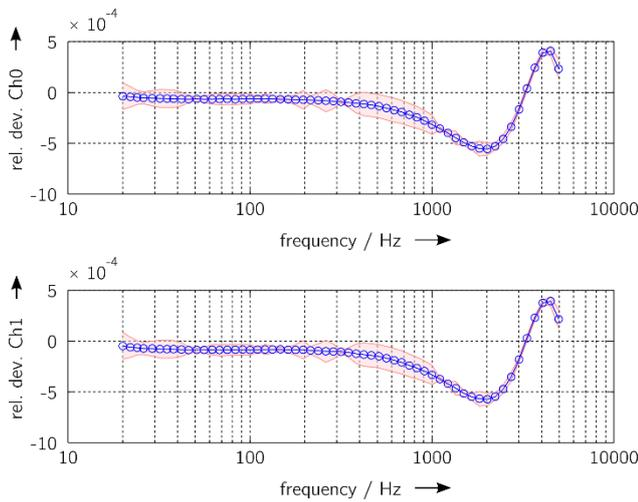
Figure 5: Calibration results for a PXI-5922 digitiser card. The relative deviations are given in blue, and the assigned measurement uncertainty  $U(k=2)$  is red. The sampling rate was 50 kS/s, and the input voltage span  $\pm 5$  V.
