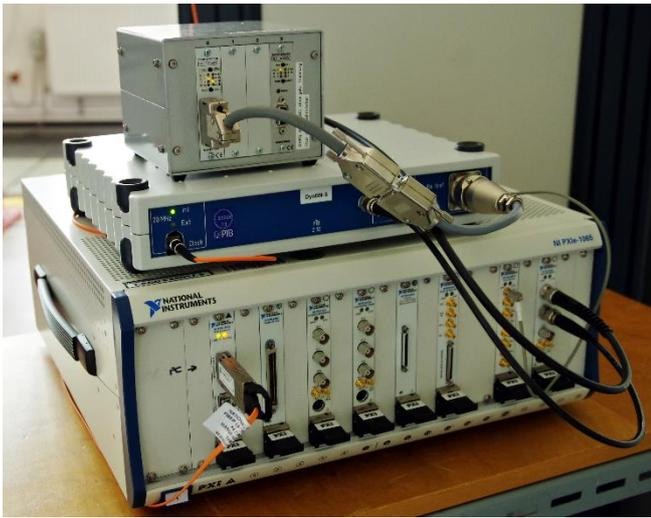
Figure 4. Dynamic bridge amplifier calibration setup, consisting of the bridge amplifier under test (top), the dynamic bridge standard (middle), and the data acquisition system (bottom).
