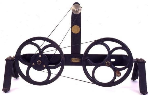
Figure 4. Colour mixer – instrument for investigating perception of colours.
