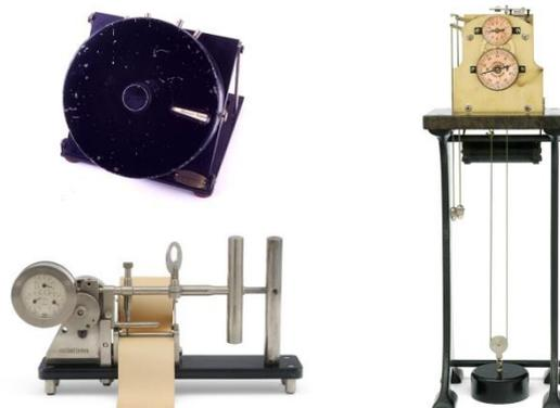
Figure 3. Old psychological instruments: Ranschburg's mnemoneter (upper left), hand ergograph after Klemm (down left), chronometer after Schultze (right).
