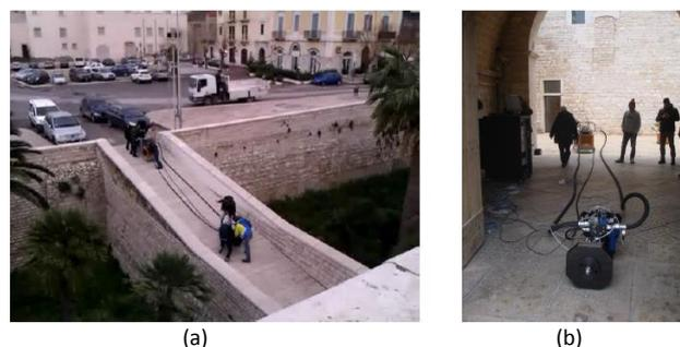
Figure 4. a) Transportation of the vibrodyne; b) Vibrodyne installed at the main entrance of the clock tower.
