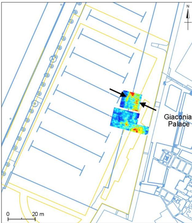
Figure 4. Lecce, sixteenth-century city fortifications: GPR time slices (147-162 cm depth; 600 MHz antenna) georeferenced in large scale map of Lecce. In yellow the layout of the “Campo Polisportivo Achille Starace”.
