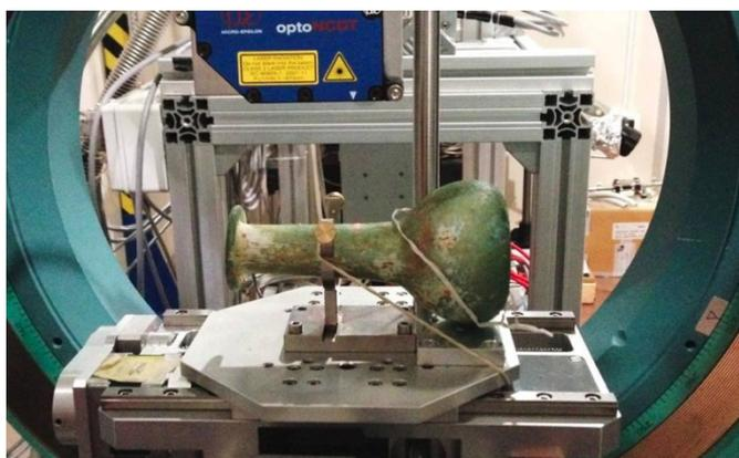
Figure 1. The diffractometer, equipped with the laser interferometer, hosting an object relevant for cultural heritage for x-ray diffraction analysis.
