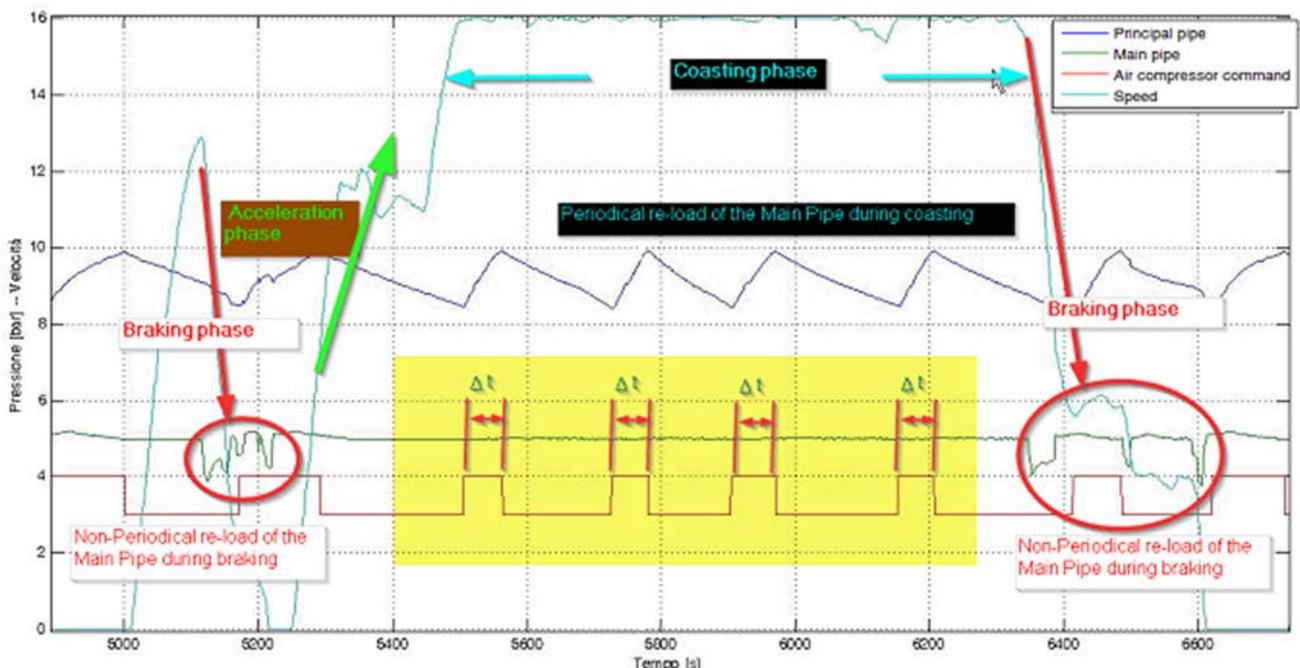
Figure 9. Typical profile of pressure and compressor operations.
