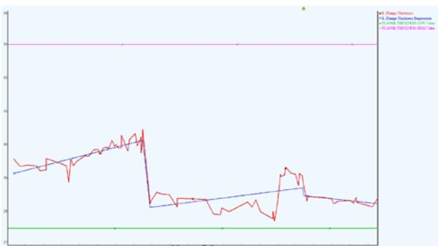
Figure 15. Flange Thickness (red line), its linear regression (blue line) and its limits (green and pink lines).
