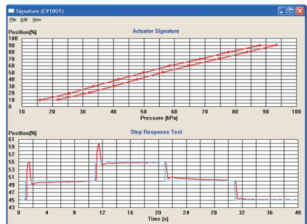
Figure 4. Example of signature for a pneumatic actuator.
