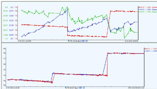
Figure 14. Top: Diameter, Flange Height and Flange Thickness trends of the same wheel; Bottom: Diameter trends of two different wheels.
