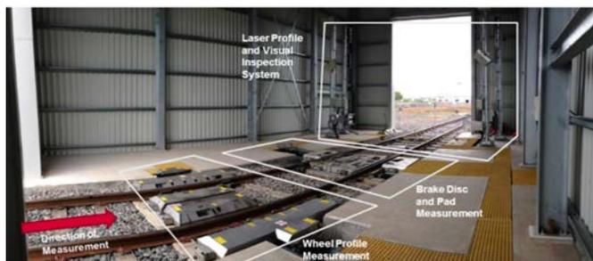
Figure 11. Vehicle Equipment Measuring System (VEMS).
