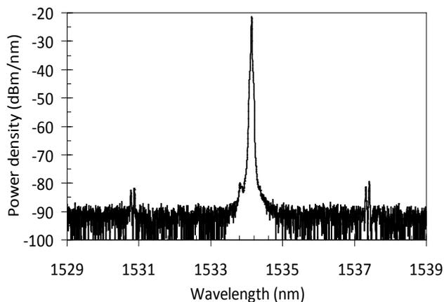
Figure 3. Measured optical spectrum of the erbium microchip laser.
