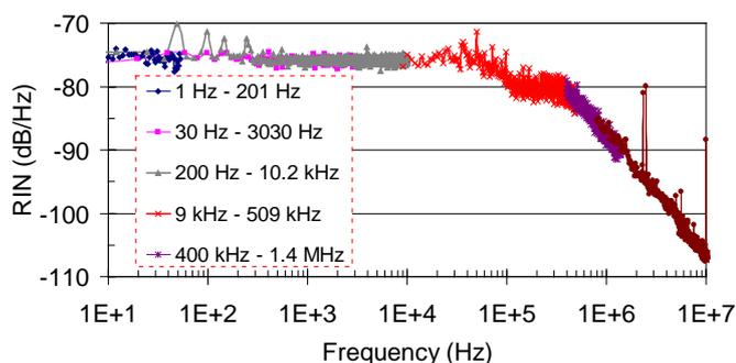
Figure 4. RIN spectral density for the pump laser.
