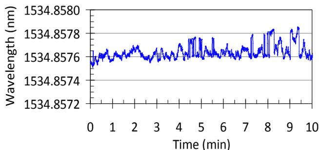
Figure 6. Laser wavelength stability over 10 minutes.
