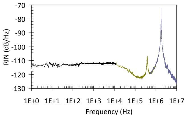
Figure 5. RIN spectral density for the Yb-Er:glass single-mode laser.
