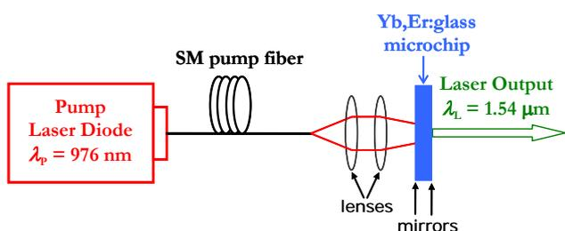
Figure 1. Set-up of fiber-pumped Yb,Er:glass microchip laser.
