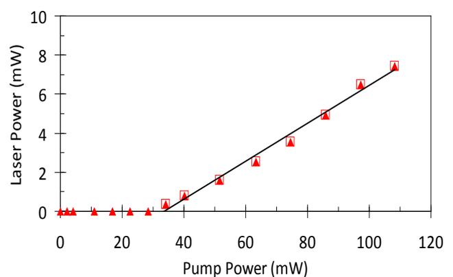
Figure 2. Measured input output laser behaviour with a linear regression of the data points above threshold showing the laser threshold and slope efficiency in single-mode operation.
