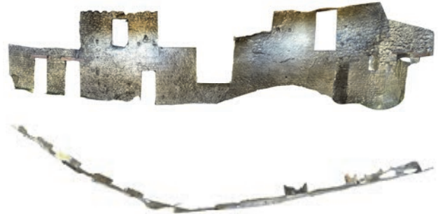
Fig. 13: Orthophoto and top view from filtered images in Recap 360 Photo.
