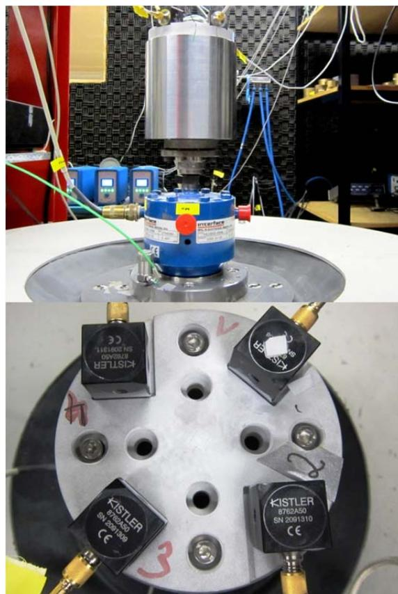
Figure 2. The upper picture shows the whole arrangement of the force transducer with the test mass, which was equipped with a special plate where four triaxial accelerometers have been mounted. The lower picture shows the plate with the four triaxial accelerometers.
