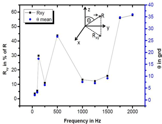
Figure 5. Vector components of the triaxial acceleration measurement. The amplitude of the transverse acceleration as well as the angle of inclination of the acceleration vector in respect to the vertical of the top mass surface (z-axis) as a function of the excitation frequency.
