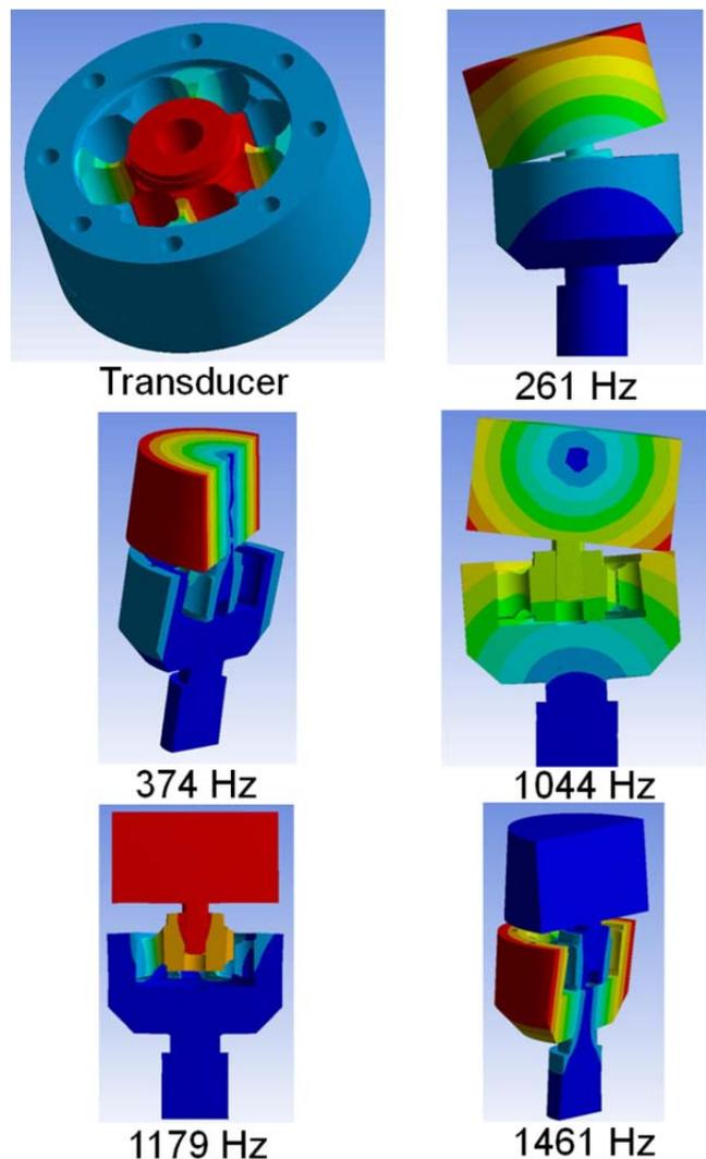
Figure 6. FEM model calculations of the force transducer equipped with a loading mass. Shown are the inner structure of the used transducer, upper left corner and the behaviour of the system at different modal frequencies. The colours give the amount of stress level whereby red indicates high stress and blue no stress.
