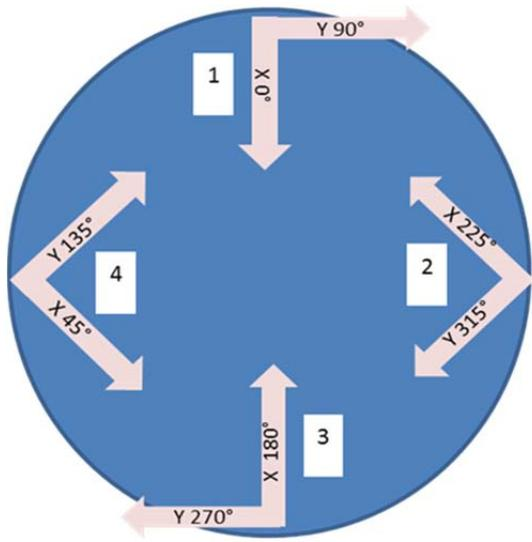
Figure 3 Schematic representation of the arrangement of the four triaxial accelerometers with their acceleration vectors in the transverse directions, x and y. In addition there are four accelerations perpendicular to the shown plane, in the z direction.
