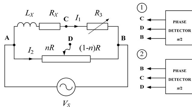
Figure 5. Diagram of the quasi-balanced bridge for loss factor measurement.
