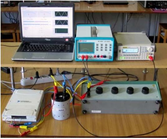
Figure 7. View of the prototype of the quality factor meter realized as the quasi-balanced circuit with dual quasi-balancing.
