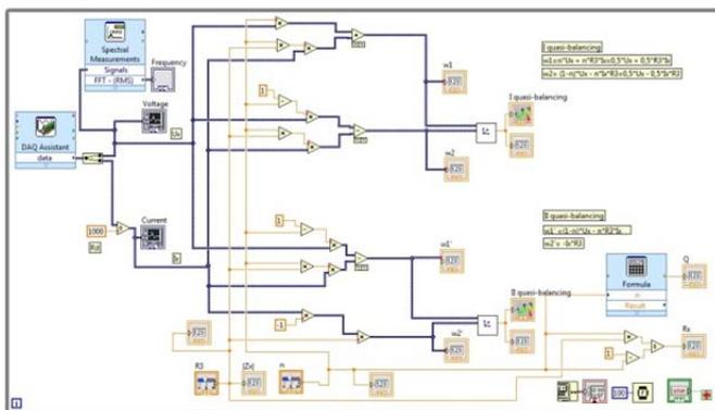
Figure 8. Block diagram of a quasi-balanced circuit with dual quasi-balancing.
