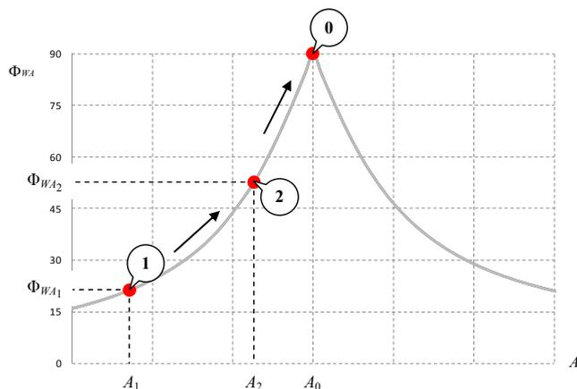
Figure 4.  $\Phi_{WA}$  signal vs. parameter  $A$  for unknown loss factor  $\text{tg } \delta_x$  values (conversion characteristic).
