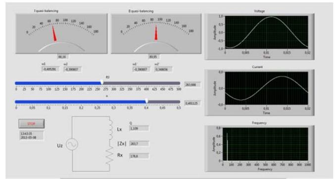
Figure 9. Front panel of a quasi-balanced meter with dual quasi-balancing.
