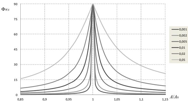
Figure 2.  $\Phi_{WA}$  signal vs. relative parameter  $A/A_0$  for different loss factor  $\text{tg } \delta_X$  values.
