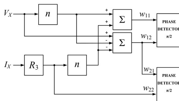
Figure 6. Block diagram of a quasi-balanced circuit with dual quasi-balancing.
