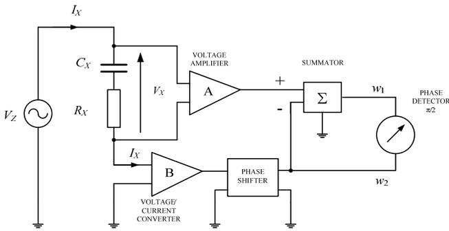
Figure 1. Block diagram of the quasi-balanced circuit for capacitance measurements.
