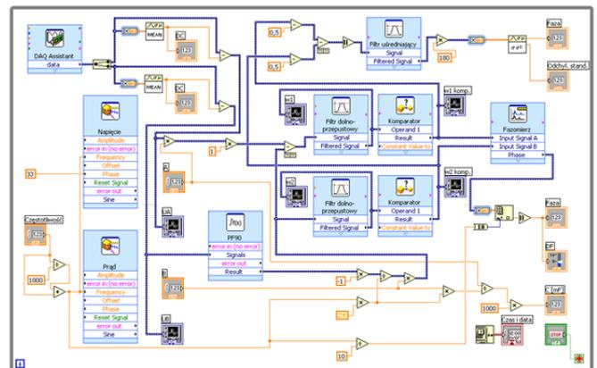
Figure 3. The LabVIEW realization of the virtual capacitance meter.
