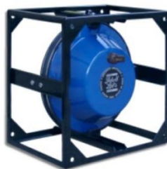
Figure 1. The sound pressure generator, Lubell model LL9642T, used as acoustic source.
