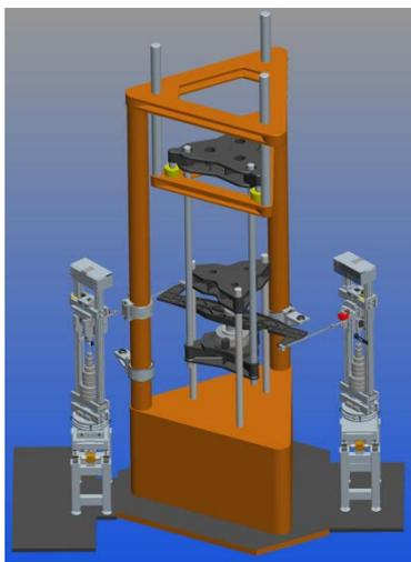
Figure 2. CAD model of the set-up of the multi-component measuring facility and additional mass stacks.
