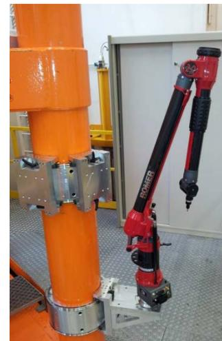
Figure 3. The figure shows the portable coordinate measuring arm, which is mounted at a pillar of the 1-MN-K-NME frame.
