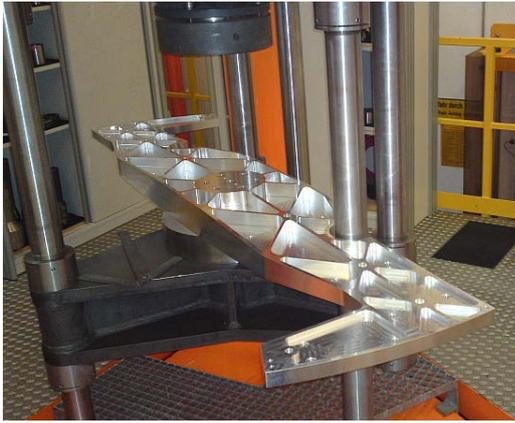
Figure 7. The figure shows the first version of the aluminium lever mounted on the 1-MN force standard machine. The shown shape has been retained for the INVAR lever. One can also see the measurement points used to determine the position towards which the coordinate measuring machine later moves.
