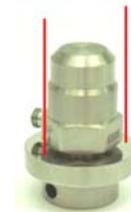
Figure 4. SE reference accelerometer mounted on top of the stainless steel mounting adapter.
