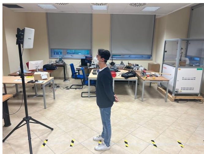
Figure 1. The simplest configuration of the system, consisting of a single RFID antenna.
