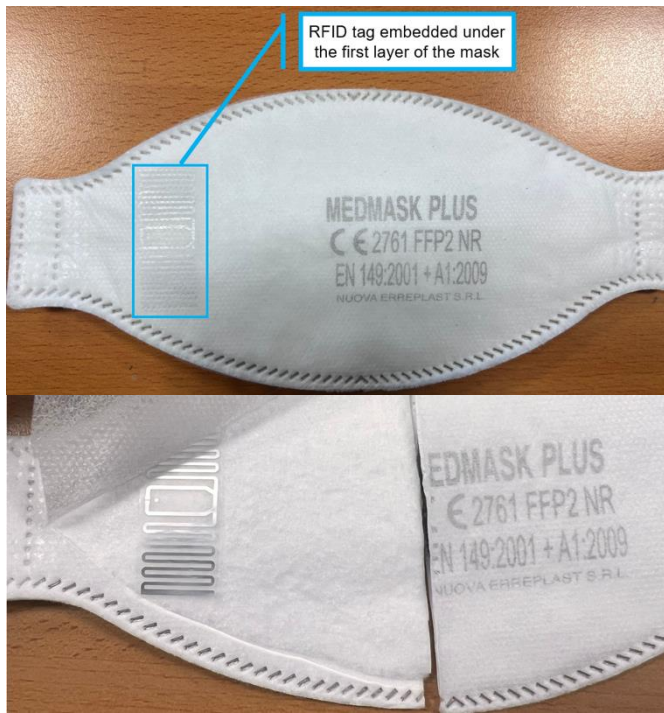
Figure 2. PPE with FFP2 filtering capacity equipped with an integrated RFID tag.
