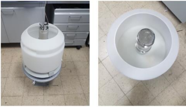
Figure 4. Mass calibration of a rainfall weighing gauge.
