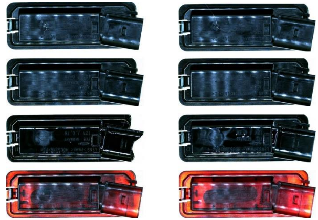
Figure 5. Style-GAN generated LED housing images showing top down: hot nozzle effects, perfect, little holding effects and effects of incorrect granulate composition.
