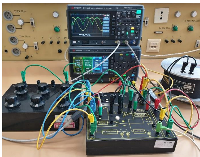
Figure 6. Measurement task: digital impedance and admittance meter prepared for remote measurement.
